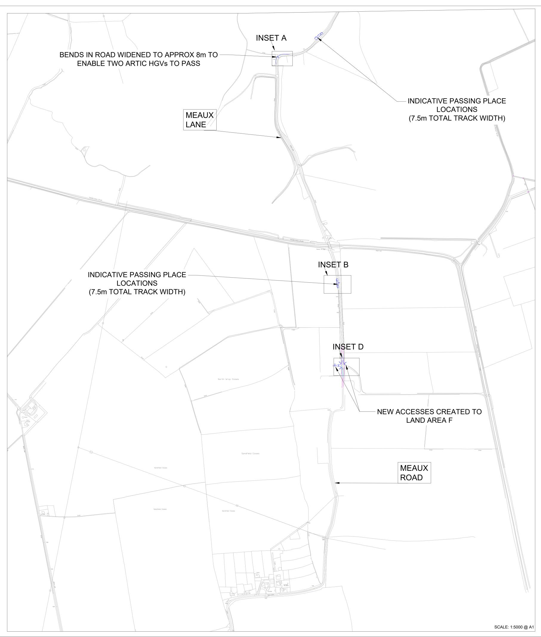
NOTES PROPOSED EDGE OF CARRIAGEWAY EXISTING 40mph VISIBILITY SPLAY (2.4m x 90.0m) PROPOSED 30mph SPEED REDUCTION VISIBILITY SPLAY (2.4m x 90.0m) FORWARD VISIBILITY SPLAY REVISIONS DATE BY DESCRIPTION 19.01.24 CGQ FIRST ISSUE A UPDATED PASSING PLACE
